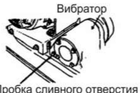
Fig-17 Vibrator Oil Plug
