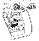
A machine that is factory equipped with a 3-speed gearbox is designed to minimize the necessary adjustments for blade size changes. However it will require some adjustments. The machine is configured from factory to operate with a specified range of blade sizes inside the factory installed blade quard.
