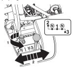
Hand tight knob. Tighten jam nut (30 ft-lb/40 Nm).
