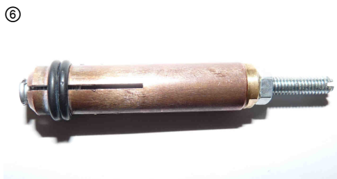
The copper base has 4 slots and is dedicated to M4 studs
