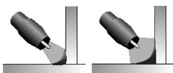
The frequency enables adjustment of the arc concentration. The higher the frequency, the more concentrated the arc. The lower the frequency, the wider the arc. In AC mode, the frequency is manually adjusted. When using AC Easy mode, this setting is automatically adjusted according to the diameter of the electrode used and welding current. It is recommended to use AC in Easy mode.
