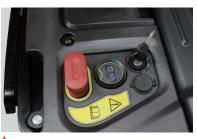
Integrated functional area, equipped with key switch, emergency switch, battery indicator and USB charging port.
