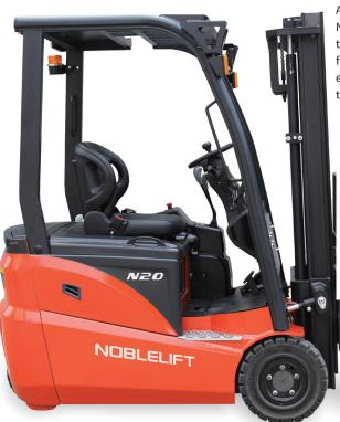
All-around Dual AC front wheel drive motors for the N series provide powerful travel and excellent turningperformance even in the most undesirable floor conditions. Stability of the truck is further enhanced through a low mounted battery, keeping the truck center of gravity lower to the ground.
