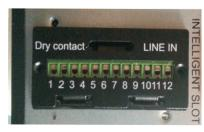
4. Connect with monitoring device by connecting wire of dry contact card. The monitoring device will display and control UPS operating status, to achieve remote monitoring of UPS operation.
