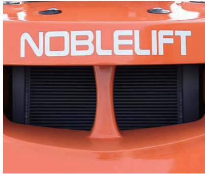
Radiator' splate fin heat dissipation system keeps engine running reliably, even in the most demanding applications.
