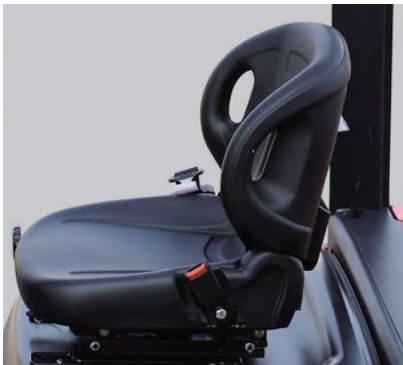
Operator Presence System (OPS) -When operator is not in seat, the hydraulic lift and tilt controls automatically lock out and traveling is disabled.
