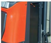
The option of side battery replacement allows customers to use the truck with multi-shift operation and not to waste time on complicated procedure of battery replacement through the top. With help of specially designed trolley, the batteries can be replaced fast and effortlessly.
