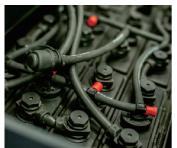
The trucks can be equipped with the option of Aquamatic- the system of fast refilling of distilled water in lead-acid batteries. The 2-ton pallet truck can be optionally equipped with the battery under 3VBS standard, which helps to reduce the length of the original truck and make it more compact (the standard battery is 2PzS)
