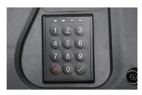
The PIN-code lock can be set with multiple passwords and also supports RFID card activation.
