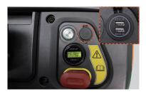
The Multi-functional LCD indicator displays the information about remaining battery power, amount of working hours and fault codes.
