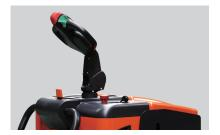
A variety of security measures such as emergency button, reverse button on tiller, and tiller push emergency stop ensure the operator's safety.
