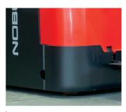
The use of apron with 8 mm thickness allows to ensure the robustness of chassis and its strength even in case of collision against objects. The strong battery cover made out of steel helps to provide a high level of strength for this part.
