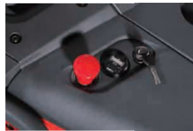
Key-switch, emergency switch and battery discharge indicator.
