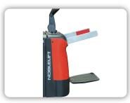
The integrated foldable ride-on platform and protective arm, as well as the new internal structure of the body, make the overall length of the stacker truck as short as possible, and achieve a smaller turning radius in the same industry. In addition, the floating structure of the ride-on platform makes the operation more comfortable.
