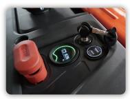
The multi-function instrument can display the vehicle working status, battery power, working time, driving speed and steering angle. When the vehicle fails, the outer ring aperture of the instrument will change from green to red, and the fault code will be displayed.
