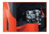
Low-noise gear hydraulic pump reduces the lifting noise of the whole vehicle.
