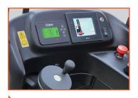
Multi-function color LCD instrument can display information such as steering wheel position, battery power, power alarm, fault code, running time, driving speed etc. The driving speeds of low, medium and high third gear can be set through the meter.
