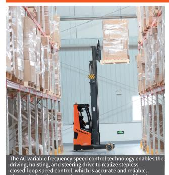
Electro-hydraulic proportional control system, good fretting performance, more stable work and more precise control.
