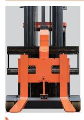
The layout of lifting cylinder and pipeline system is optimized, and the pipeline of the door frame is simple and beautiful, and the vision is excellent.
