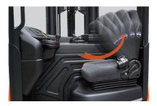
The high suspension seat greatly reduces the vibration transmission to the driver. At the same time with the automobile-type bionic curved backrest, it can effectively reduce the driver's driving fatigue. The seat can be adjusted to meet the needs of operators of different heights and shapes.
