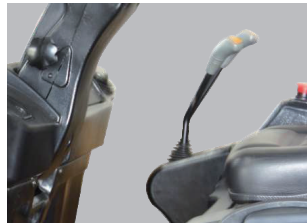
Hydraulic operating handle on the right side.
