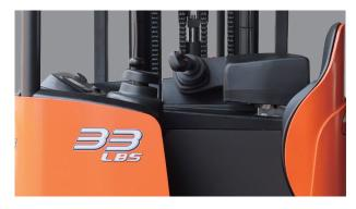
The armrest provides a 6cm/2inch adjustment range to improve the comfort of operators at different heights.
