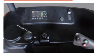
Tilt control system: can limit the tilt of the goods when the forks are high lifted to prevent roll over, and there is a one-button FORK TILT LEVELING function to ensure safety.
