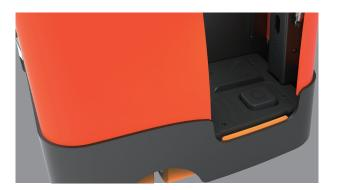
The floor suspension system adapts to the weight of the operator and provides impact and vibration protection.
