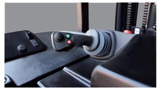
The multifunctional intergrated handle not only has lifting, lowering, tilting and side shifting, but also forward and backward shifting through the handle control, which is fast and convenient to use.
