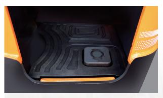
Safety protection pedal: When the operator steps down the protection pedal, the forklift will slow down.
