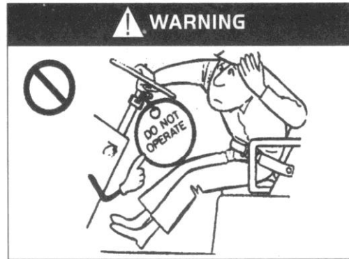
Do not drive an unsafe forklift!
