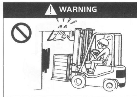
Always pay attention to the height of work place!
