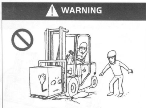
Avoid driving on soft ground, only allowed to run on solid and flat ground.
