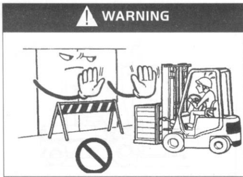
Work in specified area
