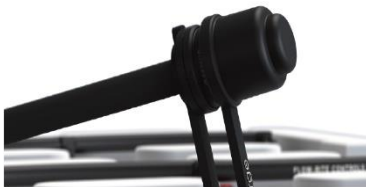
Fig.30: Replace dust cover
