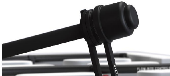
Fig.20: Place the dust cover
