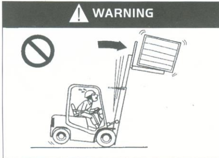
Prohibit forward tilt to enhance loading, so as to avoid tipping!
