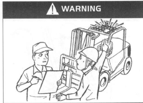
Do not drive a damaged truck!
