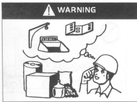
Notice the change of rated load weight before use forklift.
