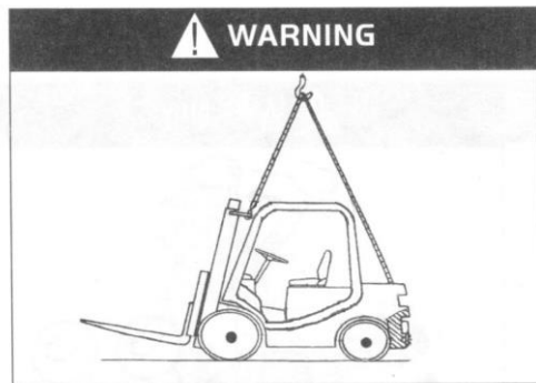
Hoisting the forklift correctly!
