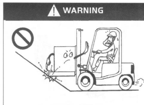
Pay attention to the steep uphill slopes and goods lifting height!
