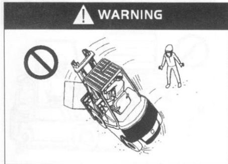
While turning a high speed can cause accident because of unstable center of gravity!
