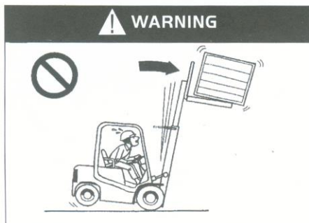
Prohibit forward tilt to enhance loading, so as avoid tipping!
