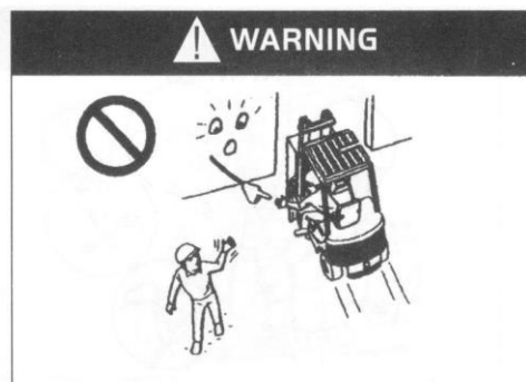
Do not put arm and body outside of the overhead guard during work!
